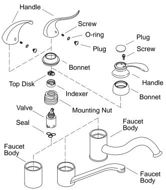
Lift off handle. Unscrew bonnet by hand. Unscrew valve mounting nut. Gently loosen and lift out valve.
