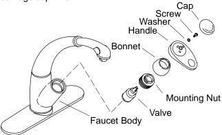
Remove screw and washer. Lift off handle. Unscrew bonnet by hand. Unscrew valve mounting nut. Gently loosen and lift out valve.
