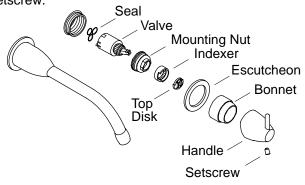
Unscrew bonnet by hand. Unscrew valve mounting nut. Gently loosen and lift out valve.
