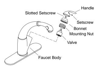
Remove the slotted setscrew from the valve stem. Unscrew the bonnet by hand. Unscrew valve mounting nut. Gently loosen and lift out valve.
